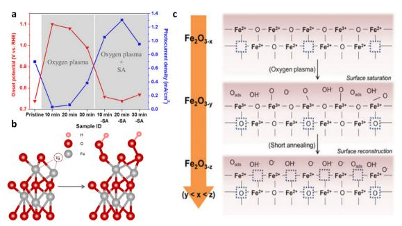
Fig. 12 Impact of oxygen plasma treatment. (a) Plasma treatment effects, with and without short annealing, on the onset potential and photocurrent density at 1.23 V<sub>RHE</sub>. (b) Formation of FeOOH on the (0001) surface of hematite as a result of oxygen plasma treatment. Reprinted with permission from ref. 110, Copyright 2016 American Chemical Society. (c) Effect of post-treatment on the hematite surface. Reproduced from ref. 111 with permission from Springer Nature, copyright 2018
