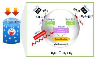
Fig. 1 PEC basics: schematics of overall water splitting
