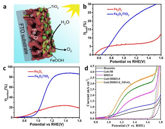
Fig. 15 Grain boundary modification by metal oxide and elemental doping. (a) Decoration of TiO<sub>2</sub> on grain boundaries. (b) and (c) Surface and bulk charge efficiency improvement by grain boundaries modification. Reproduced from ref. 124 with permission from Elsevier, copyright 2019. (d) J-V curve analysis of grain boundaries modified hematite photoanodes. Reproduced from ref. 125 with permission from Royal Society of Chemistry, copyright 2023.
