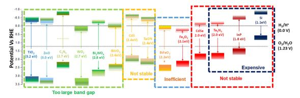
Band characteristics: band position and band gaps of different photocatalysts
