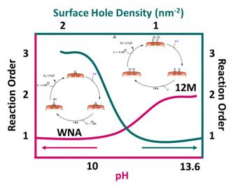
Fig. 6 Mechanism: factor affecting the rate of water splitting on hematite.
