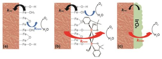
Fig. 20 Kinetic pathway for (a) hematite, (b) hematite with a molecular catalyst, and (c) hematite with a metal oxide catalyst. Reproduced from ref. 152 with permission from Royal Society of Chemistry, copyright 2023.
