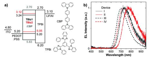
Fig. 24 (a) OLED device structure and (b) EL spectra for TBtz1 (black lines) and TBtz2 (red lines). Reproduced from ref. 130 with permission from the Royal Society of Chemistry
