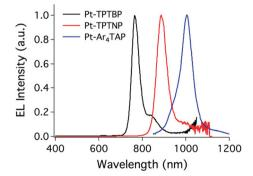
Fig. 6 Electroluminescence spectra of porphyrin platinum(II) complexes. From left: Pt-1, Pt-2, and Pt-3. Adapted with permission from ref. 35 Copyright 2011 American Chemical Society.
