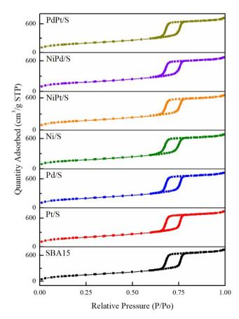
Fig. 2 N<sub>2</sub> adsorption-desorption isotherms of the SBA-15 support and calcined catalysts.
