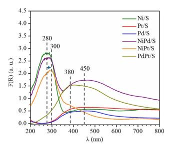
Fig. 5 UV-vis diffuse reflectance spectra of calcined catalysts.
