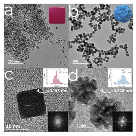
Fig. 1 TEM images of (a and c) Pt<sub>CUBE</sub> and (b and d) Pt<sub>DEND</sub>. Insets show particle size distributions and fast Fourier transform (FFT) patterns of the corresponding NPs.
