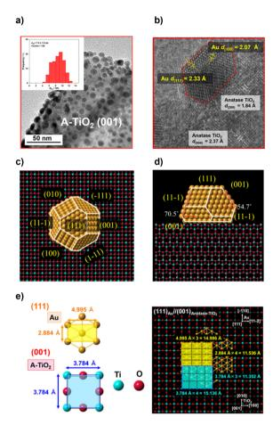
Fig. 2 TEM (a) and HR-TEM (b) images of the DP-Au/A-TiO $_2$  NPLA. Top view (c) and side view (d) of faceted Au NPs on A-TiO $_2$ (001) constructed by the Wulff theorem. (e) An interface junction model with the (111) $_{\rm Au}$ /(001) $_{\rm A-TiO}_2$  orientation.
