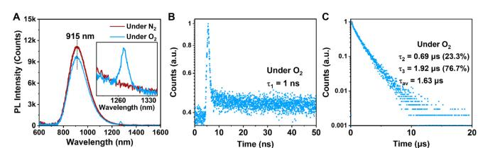
Fig. 3 (A) PL spectra of  $Au_{39}$  under  $N_2$  atmosphere (dark red line) and  $O_2$  atmosphere (blue line). Inset shows the expanded region where singlet  $O_2$  emits. (B) Decay profile measured on the 50 ns scale (measured by TCSPC). (C) Decay profile measured on the 20  $\mu$ s scale (measured by MCS).
