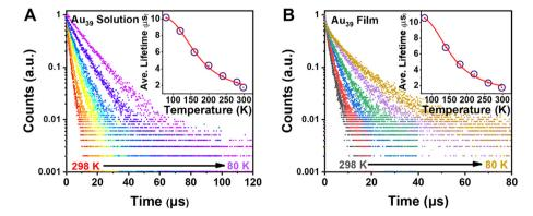
Fig. 4 (A) Temperature-dependent PL decay profiles of  $Au_{39}$  in 2-methyl-THF with excitation at 400 nm. Inset: plot of average lifetime and fitting by eqn (2). (B) Temperature-dependent PL decay profiles of  $Au_{39}$  in films. Inset: plot of average lifetime and fitting by eqn (2) (see main text).
