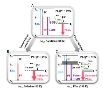
Scheme 1 Emission mechanism of Au<sub>39</sub> NCs in (A) solution (298 K), (B) solution (80 K), and (C) film (298 K).
