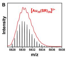
Fig. 1 (A) ESI mass spectrum of  $Au_{39}(PET)_{29}$  (CsOAc was added to facilitate ESI analysis); (B) experimental isotope pattern (red profile) of m/z at 5830.70 (corresponding to  $[Au_{39}(SR)_{29}]^{2+}$  according to the spacing of 0.5, red profile) and the theoretical pattern (black).
