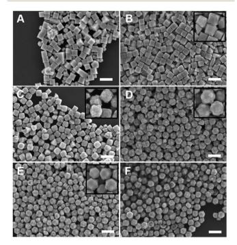
Fig. 2 SEM images of Pd nanoparticle shape as a function of iodide concentration in BioXtra CTAB. (A) 0.24, (B) 0.48, (C) 0.97, (D) 1.45, (E) 1.94, and (F) 2.90 µM added NaI in a standard growth solution that would produce THH in BioUltra A CTAB. Scale bars: 300 nm.
