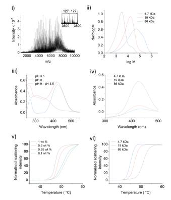
Fig. 1 (i) MALDI-MS spectra of 4.7 kDa NDA-PNIPMAM. (ii) GPC chromatograms of NDA-PNIPMAM. (iii) UV-Vis spectra of 4.7 kDa NDA-PNIPMAM at pH 3.5 and 9 with and without using the pH 3.5 spectrum as a baseline. (iv) UV-Vis spectra of different NDA-PNIPMAM polymers at pH 9 (pH 3.5 as baseline). (v) NanoDSF traces of 19 kDa NDA-PNIPMAM at different concentrations (in 10 mM TRIS, pH = 7). (vi) NanoDSF traces of different NDA-PNIPMAM polymers (0.5 mM in 10 mM TRIS, pH = 7).
