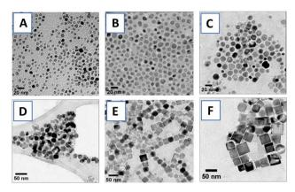
Fig. 2 Representative transmission electron microscopy (TEM) images of IONPs synthesized using thermal decomposition of Fe(acac)<sub>3</sub>: (A) 7.3  $\pm$  1.4 nm, (B) 11.0  $\pm$  2.0 nm, (C) 15.4  $\pm$  2.1 nm, (D) 19.1  $\pm$  2.3 nm nano-octahedrals, (E) 27.4  $\pm$  3.6 nm and (F) 33.4  $\pm$  4.9 nm nanocubes ( $\pm$  denotes standard deviation,  $n \ge 100$ ).
