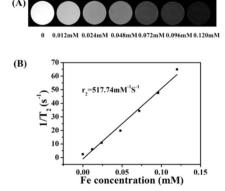
Fig. 4 (A) In vitro  $T_2$ -weighted MRI images of  $\gamma$ -Fe<sub>2</sub>O<sub>3</sub>@PNIPAM/PAm/CTS nanogels at different iron concentrations; (B) the plot of transverse relaxation rate *versus* iron concentration. The  $r_2$  value (transverse relaxivity) was calculated based on the slope of the stimulated regression lines.
