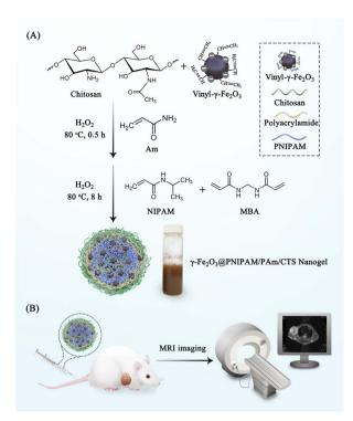
Scheme 1 (A) Illustration of the synthesis process of  $\gamma$ -Fe<sub>2</sub>O<sub>3</sub>@-PNIPAM/PAm/CTS nanogels; (B) nanogels were injected into tumor-bearing mice for MRI.
