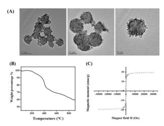
Fig. 1 (A) The TEM images of  $\gamma\text{-Fe}_2\text{O}_3$ @PNIPAM/PAm/CTS nanogels; (B) the TGA thermogram of  $\gamma\text{-Fe}_2\text{O}_3$ @PNIPAM/PAm/CTS nanogels; (C) the magnetization loop of  $\gamma\text{-Fe}_2\text{O}_3$ @PNIPAM/PAm/CTS nanogels measured by VSM analysis.
