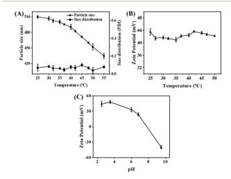
Fig. 2 Effect of solution temperature between 25 and 55 °C on (A) hydrodynamic particle size, size distribution (PDI) and (B) zeta-potential of  $\gamma\text{-Fe}_2O_3$ @PNIPAM/PAm/CTS nanogels; (C) the changes of zeta-potential of  $\gamma\text{-Fe}_2O_3$ @PNIPAM/PAm/CTS nanogels with the pH changing from acidic to alkaline condition.
