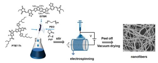
Fig. 15 The electrospinning process used to prepare D-A nanofibers. Reprinted under CC-BY 4.0 License. 48
