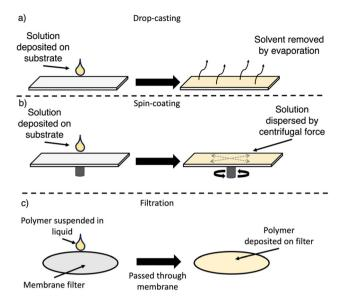
Fig. 21 Outlines of procedures used to fabricate film photocatalysts. (a) drop-casting method; (b) spin-coating method (*N.B.* spin-coating can be performed with substrate static or while spinning.); and (c) filtration.
