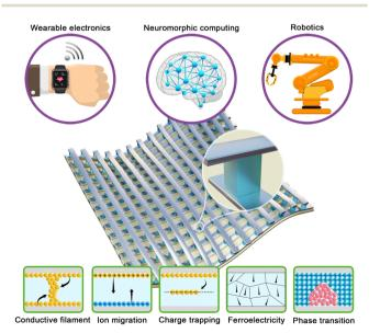
Fig. 1 Applications and mechanisms of flexible memristors.
