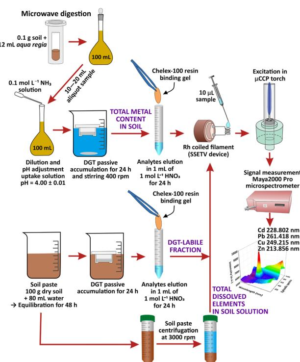
Fig. 1 Schematic diagram of soil sample preparation for the determination of total content and labile fraction of Cd, Pb, Cu and Zn in soil by SSETV- $\mu$ CCP-OES after DGT passive accumulation on Chelex-100 resin.
