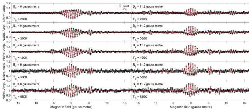
Fig. 5 Fits (red dashed line) to the experimental oscillation curves (black) measured for  $H_2$  scattering from a Cu(511) surface at a temperature of 200 K (first row), 300 K (second row), 400 K (third row), 500 K (fourth row) and 550 K (fifth row) for  $B_2 = 0$  gauss metre (left column) and  $B_2 = 11.2$  gauss metre (right column).
