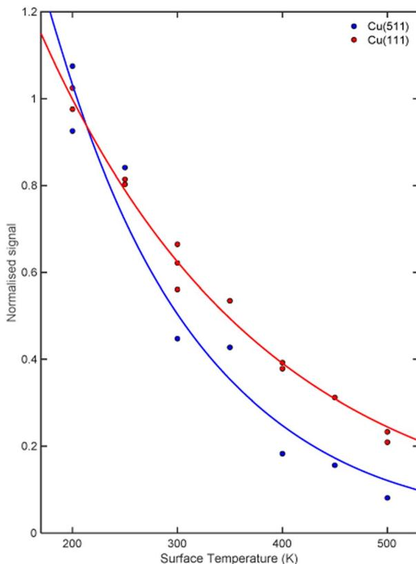
Fig. 3 Signal intensity as a function of surface temperature for the specular scattering of  $\text{H}_2$  from a Cu(511) surface (blue) and a Cu(111) surface (red) normalised with respect to the average signal intensity measured at a surface temperature of 200 K. The solid lines are exponential decay fits to the data, to guide the eye.
