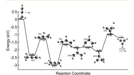
Fig. 6 Global potential energy surface of the reaction between  $Xe^+$  and propyne ( $H_3C_3H$ ) calculated at the ωb97x/aug-cc-pvtz level. All energies are shown relative to reactant energy at infinite separation, with INT1 corresponding to the first stationary point following charge transfer. Note that the allene ( $H_2C_3H_2$ ) cation is identified as INT2, and the PES for allene with  $Xe^+$  is identical to that shown here with energies being shifted to higher energies by 5 meV.
