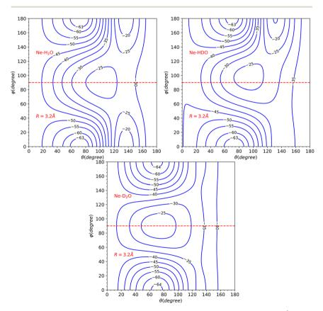
Fig. 5 Contour plots for the  $H_2O-Ne$ , HOD-Ne and  $D_2O-Ne$  PESs for R=3.2 Å. A red dashed line is placed at  $\varphi = 90^{\circ}$  to mark the symmetry of the H<sub>2</sub>O/D<sub>2</sub>O-Ne systems and the break in the symmetry of the HOD-Ne system. The labels of the contour lines correspond to the energy in cm<sup>-1</sup>.
