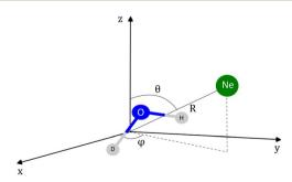
Fig. 4 Coordinates employed in the description of the HOD + Ne system. The origin of the coordinate system corresponds to the center of mass of the HDO molecule.
