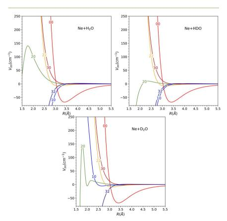
Fig. 6  $v_{lm}(R)$  expansion coefficients for the H<sub>2</sub>O-Ne, HDO-Ne, and D<sub>2</sub>O-Ne PESs. Labels in the curves are associated with lm partial waves. Only even m values are allowed for  $H_2O$ and  $D_2O$  due to the  $C_{2v}$  symmetry of these two molecules, while for HDO, even though odd m values are now allowed, just the even m values are represented to simplify the comparison.
