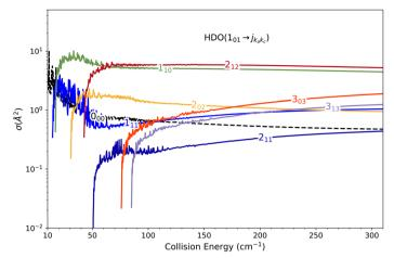
Fig. 10 Cross sections for the relaxation (black dashed line) and the excitation (solid lines) of the  $1_{01}$  rotational level of the HDO molecule by collision with Ne. Excitation cross sections correspond to transitions to the seven closest in energy excited states.
