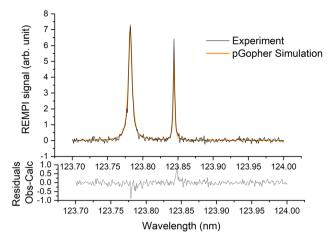
Fig. 2 Experimental (in black) and simulated (in orange) (2 + 1) REMPI spectra of the  $C^{1}B_{1}$ ,  $v' = 0 \leftarrow X^1 A_1$ , v = 0 transition of HDO in the supersonic beam. See Yang et al.<sup>21</sup> for more details.
