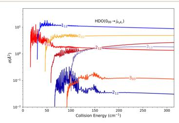
Fig. 7 Cross sections for the excitation of the fundamental rotational level of the HDO molecule by collision with Ne. The curves on the log-linear plot correspond to transitions from the  $0_{00}$  level to the first eight rotational excited states.
