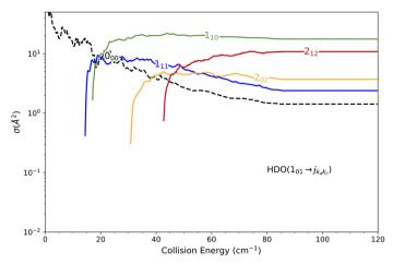
Fig. 14 Cross sections for the excitation (as solid lines) and relaxation (as a dashed line) of the first excited rotational level of the HOD molecule by collision with  $normal-H_2$ . The curves correspond to transitions from the  $1_{01}$  level to the six closest in energy rotational states
