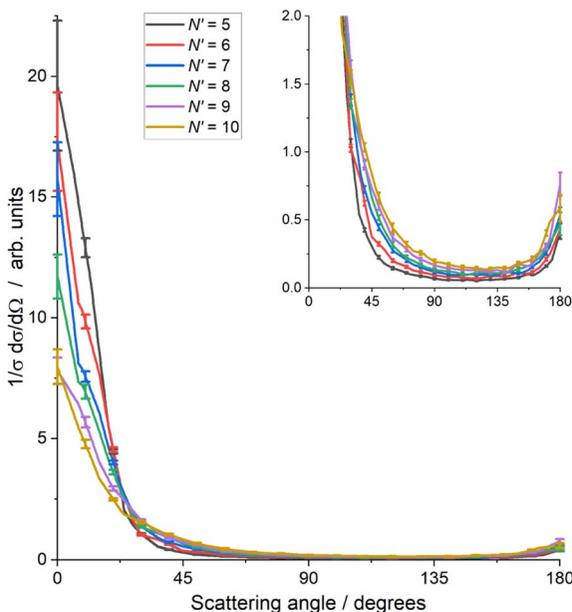
Fig. 4 Total differential cross sections, summed over all  $\text{CO}_2$  internal energies, as a function of  $\text{NO}$  final rotational state,  $N' = 5$  to 10. The inset covers a reduced vertical range to enable comparison of the sideways and backwards scattering. For each  $N'$  the integral cross section is separately normalized to unity, and the error bars represent 1 standard error.
