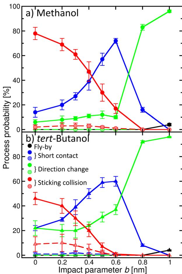
Fig. 4 Probability of the individual processes taking place in the alcohol–aqueous nitric acid cluster encounter as a function of the impact parameter  $b$ : fly-by (black), sticking (red), direction change (green), and short contact (blue). Solid/dashed lines and full/shaded symbols depict processes with/without water evaporation. Panel (a) methanol; (b) *tert*-butanol.
