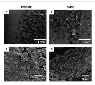
Fig. 8 SEM images of the microstructures formed on applying a 1.0 mA cm<sup>-2</sup> constant current in TEGDME (A and B) and DMSO (C and D) at two different magnifications.
