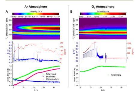
Fig. 10 Operando NMR spectroscopic measurements of Li-metal plating in symmetrical cells with 1 M LiTFSI in TEGDME under Ar (A) and O<sub>2</sub> (B) atmospheres. Spectra are plotted for the metal signals only in a shift range between 220 and 310 ppm (top) with the corresponding voltage profile and the impedance magnitude |Z| at 9 Hz (middle) and normalised intensity of the metal signal (bottom).
