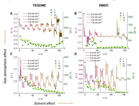
Fig. 6 The voltage traces of galvanostatic cycling for 1 M LiTFSI electrolyte in TEGDME (A and C) and DMSO (B and D), in Ar (A and B) and O<sub>2</sub> (C and D) atmospheres with currents of 0.2, 0.4, 0.8 and 1.6 mA cm<sup>-2</sup>. The I-IV labels represent different stages in the cycle: (I) nucleation, (II) surface area growth, (III) current direction switch, and (IV) plating on the opposite electrode while stripping the dendrites and stripping bulk lithium, respectively.
