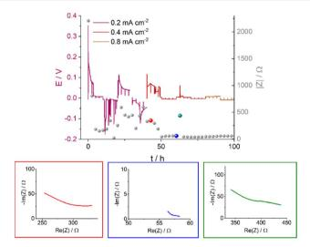
Fig. 7 The voltage traces of galvanostatic cycling for 1 M LiTFSI in DMSO in an Ar atmosphere with currents of 0.2, 0.4 and 0.8 mA cm<sup>-2</sup> (magnification of Fig. 6B) and the corresponding impedance magnitude |Z| at 9 Hz (grey balls); select Nyquist plots are shown for impedance measurements made at specific time points, illustrated by the red, blue and green balls. The red, blue and green plots correspond to before, during, and after soft shorting occurs.
