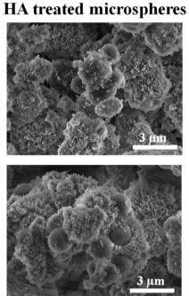
Fig. 4 SEM images of aragonite samples in the reference system and the system with untreated and HA-treated PE and PS.
