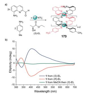
Fig. 87 (a) Subcomponent self-assembly polymerization of double helical metallopolymer 173 in the presence of a chiral solvent. (b) CD spectra showing the formation of enantiomeric helical structures as function of the enantiomeric form of the chiral solvent. Reproduced from ref. 431 with permission from the American Chemical Society, copyright 2018.
