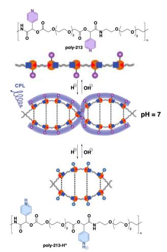
Fig. 98 Schematic illustration of double-helical AIE-active polymers 213 with multiple responsiveness via the PMPIA. Reproduced from ref. 466 with permission from the Royal Society of Chemistry, copyright 2020.
