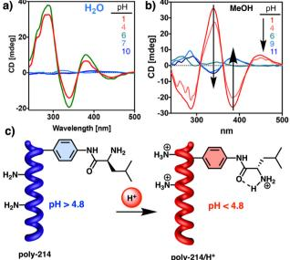
Fig. 99 CD spectra for poly-214 at different pH in (a) water and (b) MeOH. (c) Conformational composition of amino-PPAs in basic and acidic media. [amino-PPA] =  $0.5 \text{ mg mL}^{-1}$ . Reproduced from ref. 467 with permission from the American Chemical Society, copyright 2018
