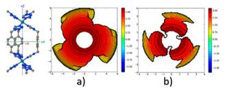
Fig. 4 Steric maps (plane xy) of the cavity of a MOF of iron, with a radius (a) 3.5 Å and (b) 6.0 Å. The centre of the MOF is at the origin, and the iron atoms are on the z axis. The isocontour curves of the steric maps are given in Å. Reproduced with permission. 148 Copyright © 2018, American Chemical Society.
