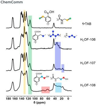
Fig. 2 Stacked solid-state <sup>13</sup>C NMR spectra of **1**-TAB, H<sub>C</sub>OF-106, H<sub>C</sub>OF-107, and H<sub>C</sub>OF-108 from top to bottom, respectively.
