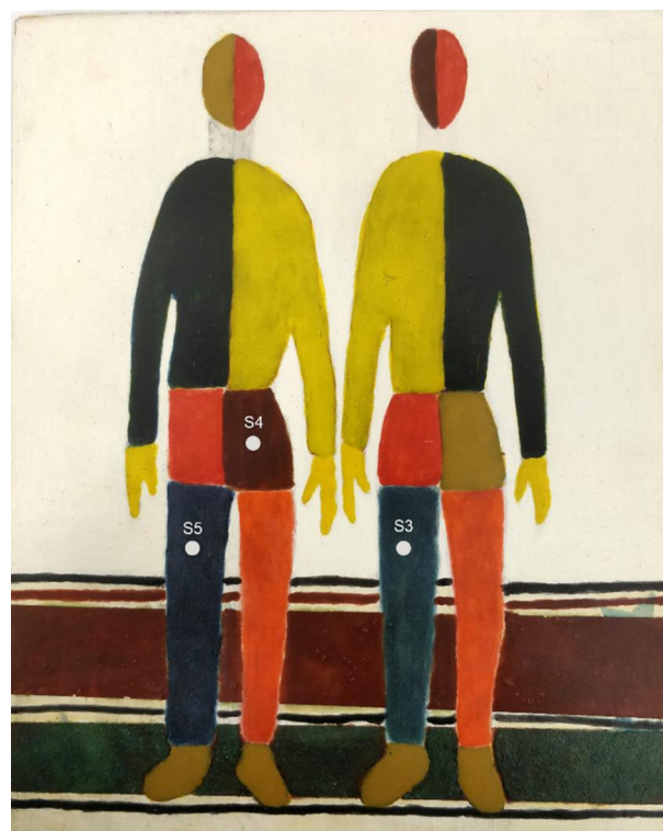
Fig. 1 Laboratory-prepared painting used to demonstrate the potential of portable fibre bundle micro-SORS coupled with serds (see ref. 22 for more details), with indication of the analysed areas (S3–S5).
