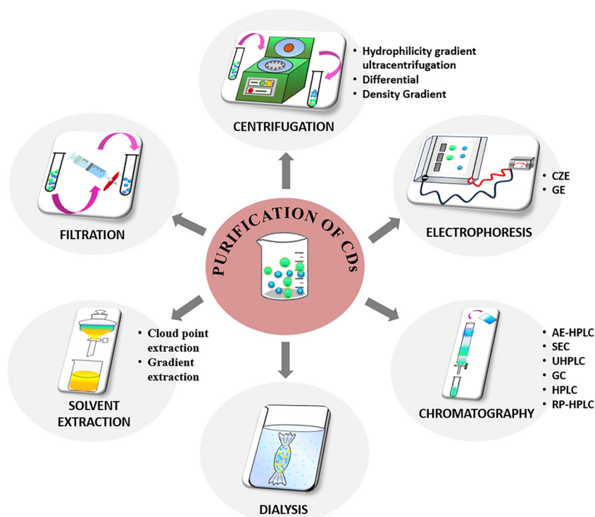
Fig. 4 Different techniques reported for the purification and separation of CDs.
