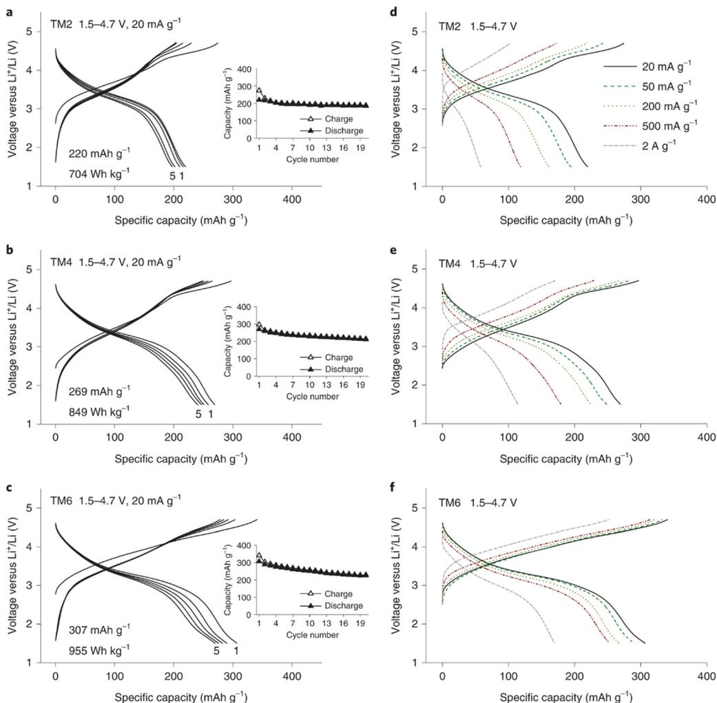
Fig. 10 Voltage curves of TM2 (a), TM4 (b) and TM6 (c) within the potential scope of 1.5–4.7 V at  $20 \text{ mA g}^{-1}$  current density (insets show the capacity retention plots), rate performance of TM2 (d), TM4 (e) and TM6 (f) exhibiting the 1st voltage curves between 1.5 and 4.7 V at 20, 50, 200, 500 and 2000  $\text{mA g}^{-1}$ . Copyright permission from Nature materials, used from ref. 146.
