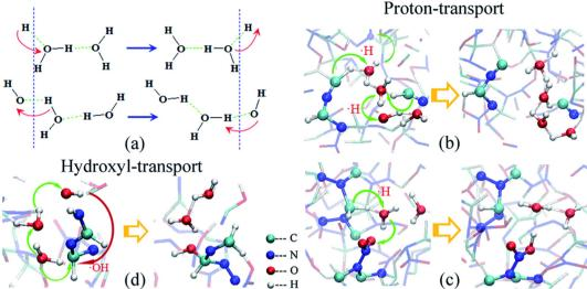
H and OH transport of water in  $\beta$ -HMX.<sup>102</sup> schematic of (a) H and OH transport, (b and c) H transport, and (d) OH transport.
