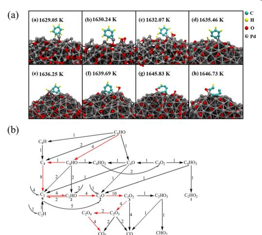
Fig. 3 (a) The oxidation process of C<sub>6</sub>H<sub>6</sub> on Pd nanoparticles and (b) further oxidation of C<sub>6</sub>HO to small molecules.<sup>54</sup>
