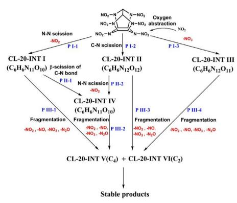
Initial pyrolysis path of the CL-20 molecule. 119
