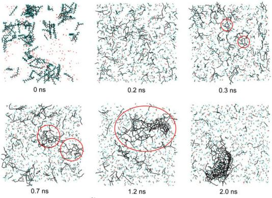
Fig. 6 Soot nanoparticle nucleation evolution process.<sup>84</sup>
