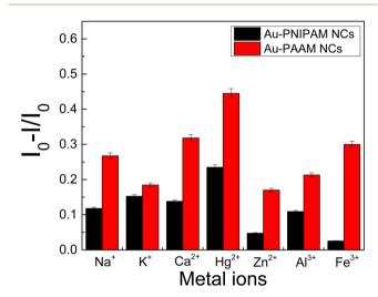
Fig. 11 Selectivity of Au-PNIPAM NCs (black bar) and Au-PAAM NCs (red bar) to  $Hg^{2+}$ . Plots of relative fluorescence intensity spectra  $[(I_0 - I)/I_0]$  of the Au-NIPAM NCs and Au-PAAM NCs in the presence of  $Hg^{2+}$  (20 nM) and various metal ions (20 nM) in water at pH: 7, incubation time 30 min.
