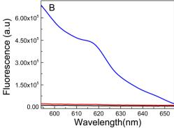
Fig. 8 Fluorescence spectra of (A) pure PNIPAM (black line), non-irradiated Au<sup>3+</sup>-PNIPAM (red line), irradiated Au-PNIPAM NCs (blue line), (B) Pure PAAM (black line), non-irradiated Au<sup>3+</sup>-PAAM (red line), and irradiated Au-PAAM NCs (blue line). Excitation wavelength: 535 nm.
