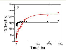
Fig. 4 Swelling kinetics of materials based on (A) PNIPAM and (B) PAAM. The profiles correspond to the materials immersed in metal precursors solutions 0.5 mM (red line) and in bidistilled water (black line).
