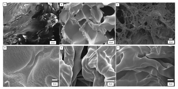
Fig. 2 SEM images of the materials: (A) PNIPAM, (B) Au<sup>3+</sup>-PNIPAM, (C) Au-PNIPAM NCs, (D) PAAM, (E) Au<sup>3+</sup>-PAAM, and (F) Au-PAAM NCs.
