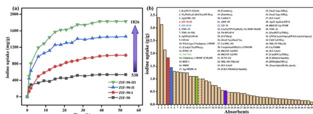
Fig. 4 (a) Iodine adsorption isotherms of ZIF-90 and ZIF-90-I-ZIF-90-III from 15 mL of  $1000 \text{ mg L}^{-1}$  iodine/cyclohexane solution, and (b) comparison of the iodine adsorption capacity from iodine solution by reported metal-organic frameworks and our materials.
