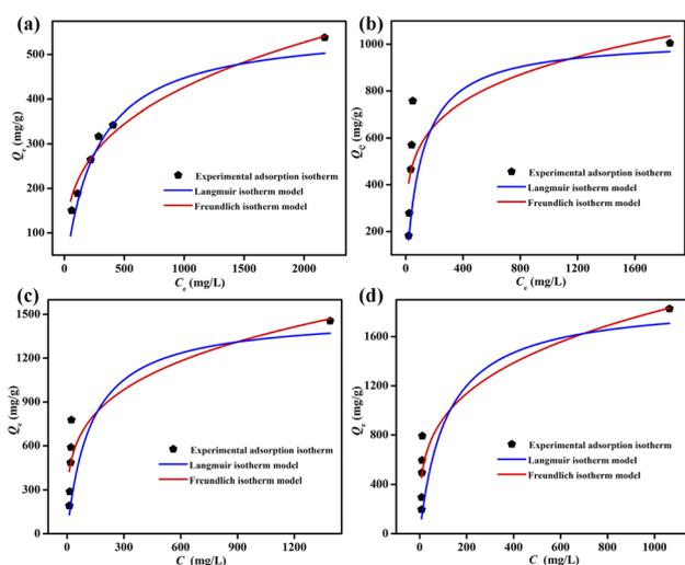
Fig. 5 The fitting of the iodine adsorption isotherms adopting the Langmuir and Freundlich isotherm models for (a) **ZIF-90**, (b) **ZIF-90-I**, (c) **ZIF-90-II** and (d) **ZIF-90-III**. High  $C_e$  values were approximately obtained using the adsorption data of 15 mL iodine/cyclohexane solution with different concentrations.
