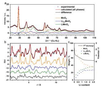
Fig. 3 (a) XRD ( $R_{\rm w}=4.5\%$ ) and (b) PDF ( $R_{\rm w}=39\%$ ) refinements of the operando data at Li 2.0. Calculated patterns from MnO<sub>2</sub> ( $P4_2/mnm$ , orange), Li<sub>0.5</sub>MnO<sub>2</sub> (Cmmm, blue) and DRX-LiMnO<sub>2</sub> (C2/m, green) are shown for comparison. (c) The change of their phase ratios during the "insertion" step derived from the PDF refinement.
