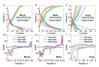
Fig. 6 The first 11 "insertion" cycles of (a)  $\alpha$ -Mn<sub>2</sub>O<sub>3</sub>, (b)  $\beta$ -MnO<sub>2</sub>, and (c)  $\alpha$ -Fe<sub>2</sub>O<sub>3</sub>. The selected derivatives of the 1st (red), 2nd (blue) and 10th (green) cycles are shown below for (d)  $\alpha$ -Mn<sub>2</sub>O<sub>3</sub>, (e)  $\beta$ -MnO<sub>2</sub>, and (f)  $\alpha$ -Fe<sub>2</sub>O<sub>3</sub>. Black arrows indicate the reversible redox pairs.
