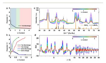
Fig. 1 (a) The 1st discharge voltage curve of MnO $_2$  cycled under C/15. Mechanistically distinct regions are highlighted using different colours. (b) First two cycles within the "insertion" regime. Black crosses mark where the cycled samples were collected for  $ex\ situ\ XRD/PDF$ . (c) XRD and (d) PDF data within the "insertion" regime, acquired from the operando X-ray total scattering experiments. Calculated Bragg peaks from  $\beta$ -MnO $_2$  and DRX-LiMnO $_2$  are shown for reference.
