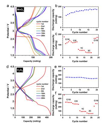
Fig. 8 (a) Selected discharge and charge cycles of DRX-LiMnO<sub>2</sub> (derived from the nanostructured  $\beta$ -MnO<sub>2</sub>), and its (b) capacity retention (under C/10) and (c) rate capability. (d) Selected discharge and charge cycles of DRX-Li<sub>3</sub>V<sub>2</sub>O<sub>5</sub> (derived from the commercial  $\alpha$ -V<sub>2</sub>O<sub>5</sub>), and its (e) capacity retention (under C/5) and (f) rate capability.
