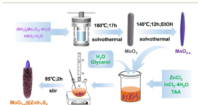
Scheme 1 Schematic illustration for the preparation of the MoO 3-x @ZnIn 2 S 4 composites.
