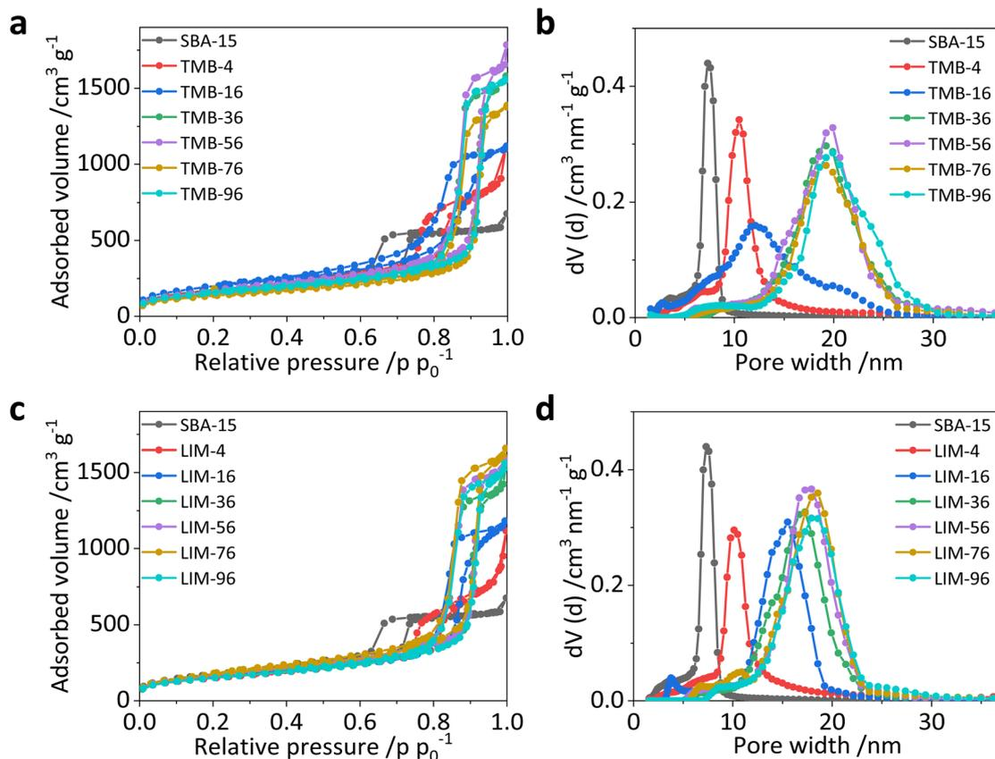
Fig. 3  $N_2$  physisorption data for varying amounts of TMB (top row) and limonene (LIM, bottom row) expander. The isotherms for samples synthesised using (a) TMB and (c) limonene are all of type IVa. The pore size distributions in (b) and (d) show a gradual increase in pore size with increasing expander to P123 molar ratio.
