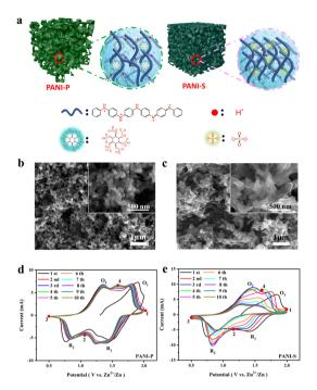
Fig. 1 (a) Microscopic schematic diagram of different PANI doped acids; scanning electron microscopy images of different PANI doped acids: (b) doped phytic acid; (c) doped sulfuric acid; cyclic voltammetry curve (CV curve) sweep rate of 10 mV s<sup>-1</sup> for different PANI doped acids: (d) PANI doped phytic acid electrode in 1 M zinc sulfate electrolyte with addition of zinc phytate (1%); (e) PANI doped sulfate electrode in 1 M zinc sulfate electrolyte.
