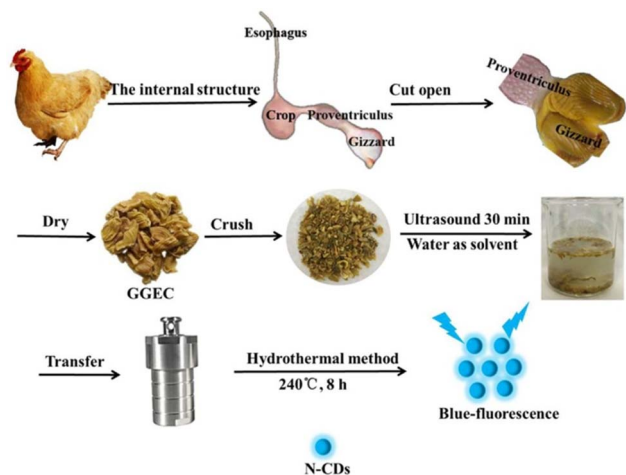
Fig. 6 A systematic diagram of N-CDs derived from GGEC by the HT method. Reprinted from ref. 216, Copyright (2021), with permission from Elsevier.
