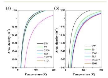
Fig. 2 The areal density of various defects versus temperature for (a) α-antimonene and (b) phosphorene. The defects considered include SW, SV-(5|9), SV-(55|66), DV-(5|8|5), DV-(555|777) and DV-(4|10|4).
