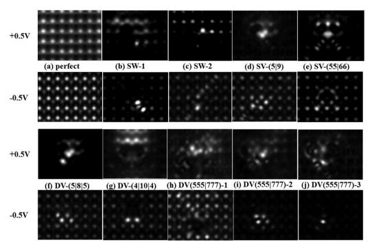
Fig. 6 Simulated STM image of the perfect  $\alpha$ -antimonene (a) and defective  $\alpha$ -antimonene with defect: (b) SW-1; (c) SW-2; (d) SV-(5|9); (e) SV-(55|66); (f) DV-(5|8|5); (g) DV-(4|10|4); (h) DV-(555|777)-1; (i) DV-(555|777)-2; (j) the simulated STM image of DV-(555|777)-3 at a distance of 2 Å from the surface.
