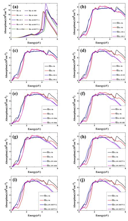
**Fig. 5** (a) Computed optical absorption coefficient in the *z* direction (perpendicular to the plane) of the perfect α-antimonene; absorption coefficient in the *x* and *y* direction (parallel to the plane) of α-antimonene with defects: (b) SW-1; (c) SW-2; (d) SV-(5|9); (e) SV-(55|66); (f) DV-(5|8|5); (g) DV-(4|10|4); (h) DV-(555|777)-1; (i) DV-(555|777)-2; and (j) DV-(555|777)-3.
