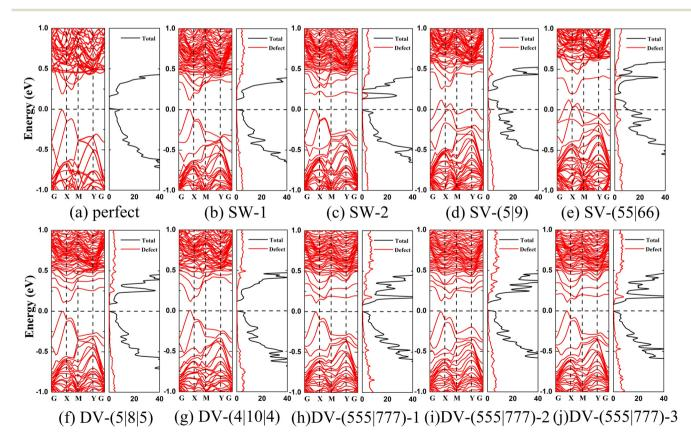
Fig. 4 Computed electronic band structure and density of states of various  $\alpha$ -antimonenes without or with defects: (a) perfect;  $\alpha$ -antimonene with defects of (b) SW-1; (c) SW-2; (d) SV-(5|9); (e) SV-(55|66); (f) DV-(5|8|5); (g) DV-(4|10|4); (h) DV-(555|777)-1; (i) DV-(555|777)-2; and (j) DV-(555|777)-3.
