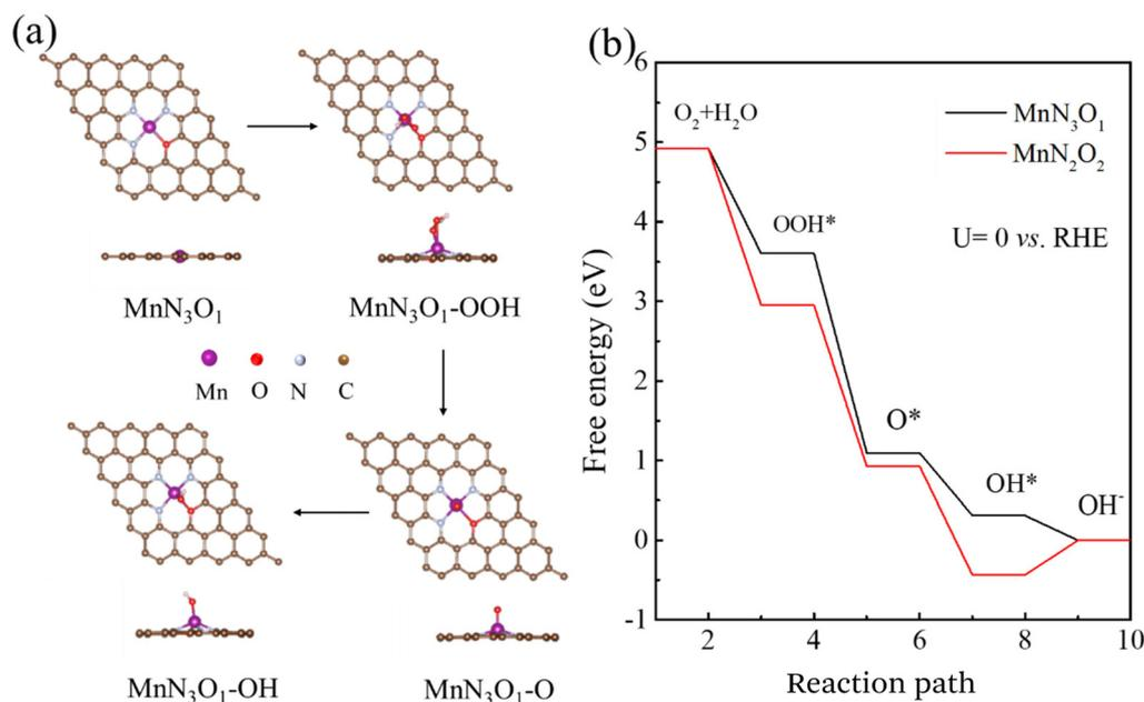
**Fig. 6** Top and side views of the optimized adsorption model of  $O^*$ ,  $OH^*$ , and  $OOH^*$  on  $MnN_3O_1$ . Brown, purple, red, and white balls represent C, Mn, O, and N, respectively. (b) Under the condition of  $U = 0$  V, the  $4e^-$  association pathway at the active site of  $MnN_3O_1$  and  $MnN_2O_2$  calculates the free energy evolution of the ORR.
