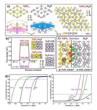
Fig. 3 (a) Graphical models to show the lattice match between NiPS<sub>3</sub> and  $Ni_2P$ ; (b)  $\Delta G_{H^*}$  calculation; (c) charge density distribution at the interface, The Ni, S, P, and H atoms are marked in gray, yellow, purple, and blue, respectively; LSV curves of (d) HER and (e) OER. Reproduced with permission from ref. 44. @ American Chemical Society, 2019.
