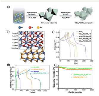
Fig. 6 (a) Synthetic process of the NiSe<sub>2</sub>/Ni(OH)<sub>2</sub> heterostructure; (b) cartoon of the heterointerface; (c) GCD curves of different catalysts; reproduced with permission from ref. 45. © Springer Nature, 2020. (d) GCD curves at 10 mA cm<sup>-2</sup> and (e) 2000 GCD cycles of the NiSe/  $Ni_3S_2/Ni_{12}P_5$  heterostructure and control samples. Reproduced with permission from ref. 42. © Elsevier, 2018.
