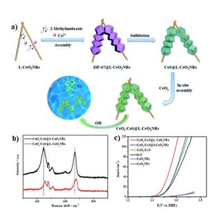
Fig. 2 (a) Scheme of the fabrication process of CeO<sub>x</sub>/CoS@L-CeO<sub>2</sub>-NRs; (b) Raman spectra of CeO<sub>x</sub>/CoS@L-CeO<sub>2</sub>NRs and CeO<sub>x</sub>/CoS@S-CeO<sub>2</sub>NRs; (c) LSV curves of different electrocatalysts. Reproduced with permission from ref. 63. © Royal Society of Chemistry, 2019.
