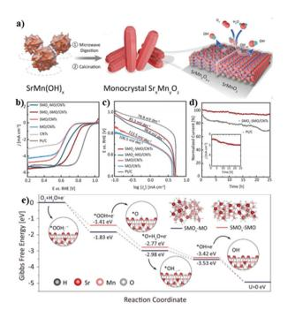
Fig. 5 (a) Scheme for the fabrication of  $SMO_x-SMO$ ; (b) LSV curves; (c) Tafel slopes and (d) chronoamperometric curves for different catalysts; (e) Gibbs free energy change chart for SMO<sub>x</sub>-SMO and SMO<sub>x</sub>-MO. Reproduced with permission from ref. 43. © Wiley-VCH GmbH, 2021.
