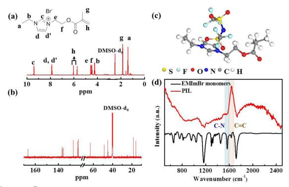
Fig. 2 (a) <sup>1</sup>H NMR and (b) <sup>13</sup>C NMR spectra of EMEImBr monomer, (c) chemical configuration of PIL, (d) FTIR spectra of EMEImBr monomer and PIL polymer matrix.
