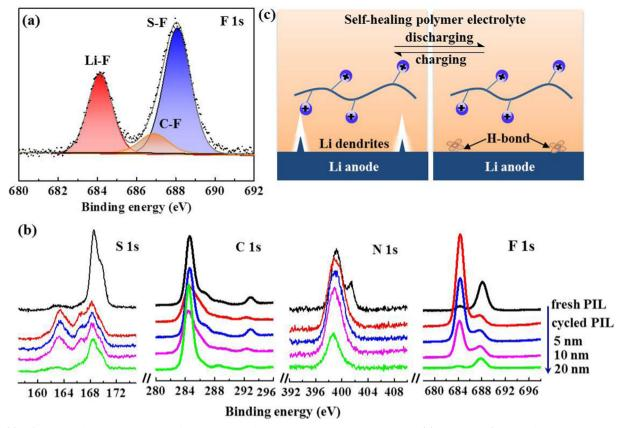
Fig. 5 (a) XPS spectra of F1s revealing the surface chemistry of cycled Li anode with PIL electrolyte; (b) in-depth XPS spectra for the PIL electrolyte after cycling; (c) schematic illustration presenting the inhibition mechanism of Li dendrites in the self-healing electrolyte.
