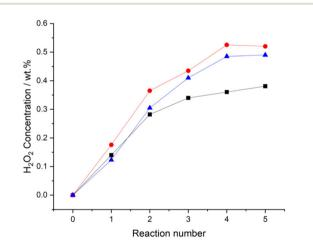
Fig. 3 Comparison of catalytic activity, over sequential H<sub>2</sub>O<sub>2</sub> synthesis reactions. Key: 0.5%Pd/TiO<sub>2</sub> (black squares), 0.25%Pd-0.25%Au/TiO<sub>2</sub> (red circles), 0.25%Pd-0.25%Sn/TiO<sub>2</sub> catalysts (blue triangles) H<sub>2</sub>O<sub>2</sub> direct synthesis reaction conditions: catalyst (0.01 g), H<sub>2</sub>O (2.9 g), MeOH (5.6 g), 5% H<sub>2</sub>/CO<sub>2</sub> (420 psi), 25% O<sub>2</sub>/CO<sub>2</sub> (160 psi), 0.5 h, 20 °C, 1200
