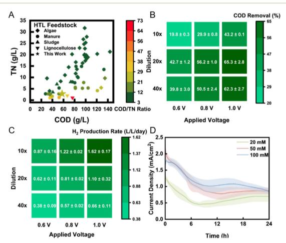
Fig. 1 (A) COD/TN composition of feedstock PHW used in this study and other PHW studies. Literature data were collected from Watson *et al.* (2020).<sup>27</sup> The COD removal (B) and H<sub>2</sub> production rate (C) of PHW-fed MEC in 3-day period under different applied voltage and dilution ratio. (D) The current density profile under different buffer strength after introduction of fresh electrolyte. The shadows represent standard deviation from triplicate experiments.
