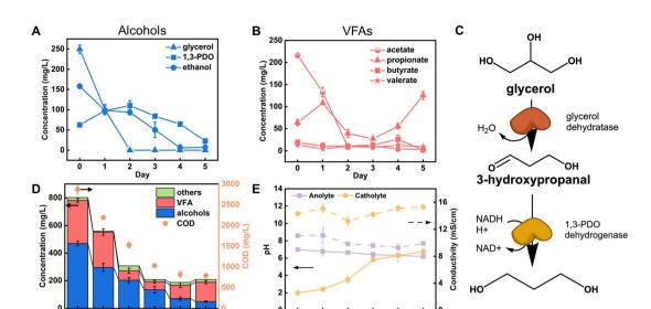
Fig. 2 The concentration profile of (A) alcohols and (B) VFAs throughout the MEC treatment as identified by HPLC with an ion-exclusion column. (C) The metabolic pathway of glycerol fermentation to 1,3-PDO. (D) The combined concentration profile of HPLC identified chemicals and the COD degradation profile. (E) The pH and conductivity change of electrolyte throughout the MEC treatment. pH is presented by solid lines and conductivity by dashed line.
