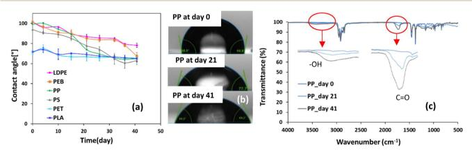
Fig. 3 (a) Changes in contact angle over 41 days of accelerated weathering. Contact angle values are expressed as average quantities  $\pm$  standard deviations from analysing three different subsamples for each sample (n=3), (b) photos of contact angle droplets produced by PP after days 0, 21 and 41 of the trial and (c) FTIR spectra for PP after the same time periods.
