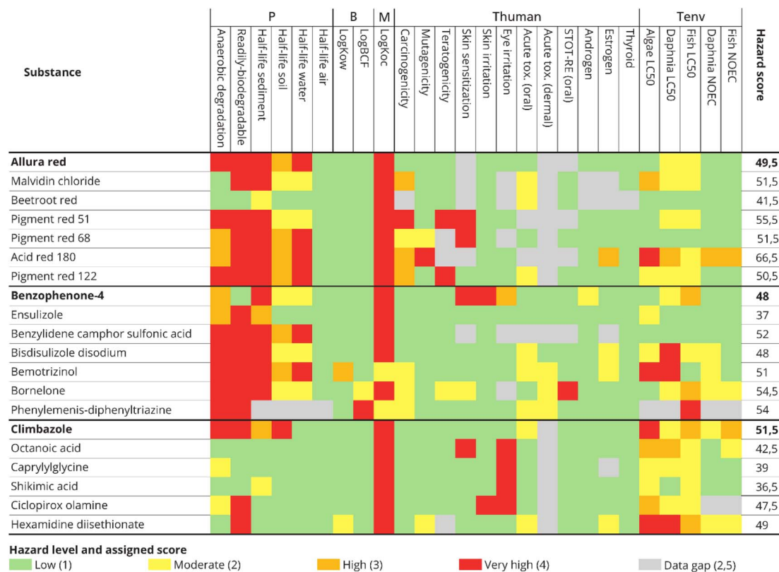
Fig. 4 Heat map and total hazard score of the three case-study chemicals and their potential alternatives for the P (persistence), B (bioaccumulation), M (mobility), human toxicity ( T_{\text{human}} ) and ecotoxicity ( T_{\text{env}} ) endpoints. The thresholds for the colour codes were based on ref. 34 and the scores were based on ref. 25. Colour codes indicate whether a hazard criterion is exceeded according to current regulatory standards and a very high hazard (red) is assigned. When hazard criteria fell below regulatory standards a high (orange), moderate (yellow) or low (green) hazard level is assigned. Chemicals with lower hazard scores compared to the case-study chemical are potentially safer alternatives.
