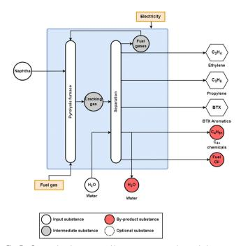
Fig. 3 Conventional steam cracking process to produce ethylene, propylene, and BTX aromatics from naphtha. The pyrolysis furnace converts the feedstock, here, naphtha, into cracking gas, which is then sent to a series of separation units to separate the various hydrocarbon fractions and waste water. Additional feedstocks for the steam cracking process include ethane, propane, butane, and gas oil. Adapted from Xiang et al.<sup>25</sup>
