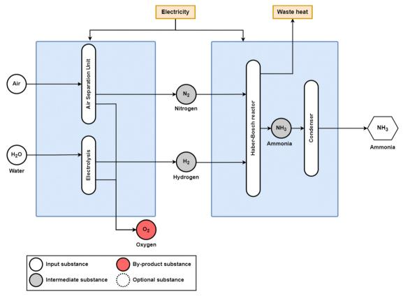
Fig. 11 Power-to-ammonia process diagram with nitrogen supplied from an ASU and hydrogen supplied from electrolysis. Adapted from Smith et al.<sup>11</sup> and Morgan<sup>55</sup>
