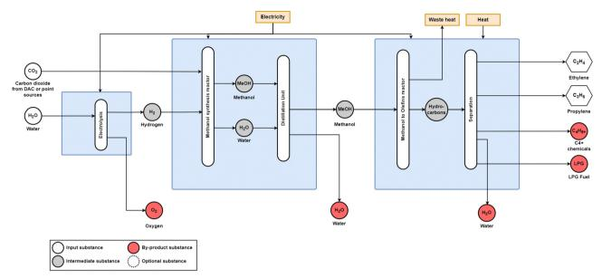
Fig. 13 Power-to-methanol-to-olefins process diagram. Methanol synthesis occurs over a CuOZnO/Al<sub>2</sub>O<sub>3</sub> catalyst and the MTO reactor uses the SAPO-34 catalyst. Adapted from Jiang et al.<sup>25</sup> and Dimian and Baldea.<sup>75</sup>
