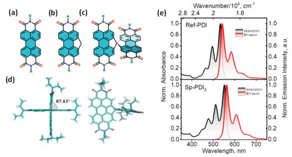
Fig. 17 Molecular structures of (a) PDI, (b) Ref-PDI and (c) Sp-PDI<sub>2</sub> (R-3-pentyl group), (d) single crystal X-ray structure of Sp-PDI<sub>2</sub>, and (e) normalized absorption (black trace) and emission (red trace) spectra of Ref-PDI (top) and Sp-PDI<sub>2</sub> (bottom) in toluene at room temperature. Reproduced from ref. 72 with permission from the American Chemical Society, copyright 2023.
