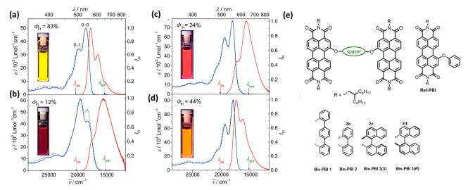
Fig. 8 Absorption (blue solid line), emission (red solid line) and excitation (green dotted line) spectra of (a) Ref-PBI, (b) Bis-PBI 2, (c) Bis-PBI 2 and (d) Bis-PBI 3(S) in 1,1,2,2-tetrachloroethane (TCE) at room temperature, and (e) molecular structures of Ref-PBI, Bis-PBI 1, Bis-PBI 2, Bis-PBI 3(S) and Bis-PBI 3(R). Reproduced from ref. 67 with permission from the American Chemical Society, copyright 2023.
