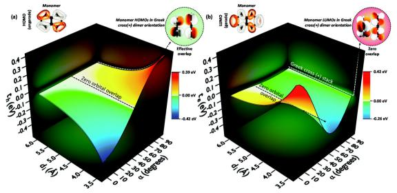
Fig. 16 (a) Hole transfer coupling  $(t_p)$  and (b) electron transfer coupling  $(t_p)$  of a naphthalene dimer with variation in the rotational angle  $(\alpha)$  and interplanar distance (d<sub>i</sub>). Reproduced from ref. 70 with permission from the Royal Society of Chemistry, copyright 2023.
