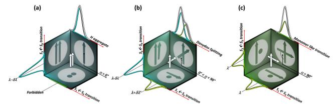
Fig. 1 Schematic representation of two transition dipoles arranged in (a) parallel (rotational angle,  $\alpha = 0^{\circ}$ ), (b) cross ( $0^{\circ} < \alpha < 90^{\circ}$ ), and (c) Greek-cross ( $\alpha = 90^{\circ}$ ) orientations with corresponding characteristics in the absorption spectra.
