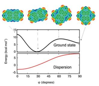
Fig. 5 Dimer geometries and potential energy curve of the electronic ground state of the geometries (black line) as a function of torsion angle  $(\phi)$ . The dispersion contribution to the total energy as a function of the torsion angle is shown in the red trace. Reproduced from ref. 66 with permission from the American Chemical Society, copyright 2023.
