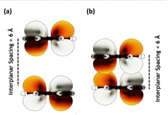
Fig. 3 MOs with (a) large (≥ 6 Å) interplanar spacing having no orbital overlap and (b) lower ( $\leq 6$  Å) interplanar spacing showing orbital overlap.
