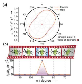
Fig. 13 (a) Anisotropic mobility computed along the ac plane and (b) schematic depiction of charge filtering demonstrating selective hole transfer in Greek (+) cross PTE-Br<sub>2</sub>. Reproduced from ref. 71 with permission from Wiley-VCH, copyright 2023.
