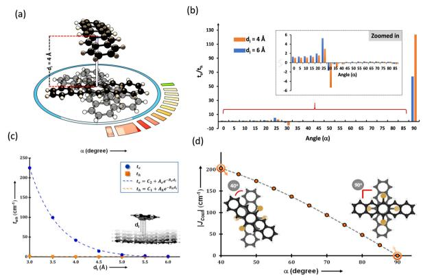
Fig. 15 (a) Greek cross (+) pentacene with intermolecular distance and angular rotation marked, (b)  $t_{\rm e}/t_{\rm h}$  with varied rotational angle, (c) graph showing the dependence of charge transfer coupling to the interplanar distance and (d) Coulombic coupling variation with respect to the rotational angle. Reproduced from ref. 74 with permission from the American Chemical Society, copyright 2023.
