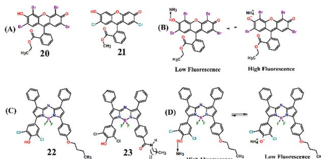
**Fig. 14** (A) Molecular structure of fluorescent indicator dyes **20** and **21** and (B) their proposed fluorescence sensing mechanism of detection of  $\text{NH}_3$  through acid–base equilibrium. (C) Molecular structure of aza-BODIPY sensors **22** and **23** and (D) their proposed fluorescence sensing mechanism of detection of  $\text{NH}_3$  through acid–base equilibrium.
