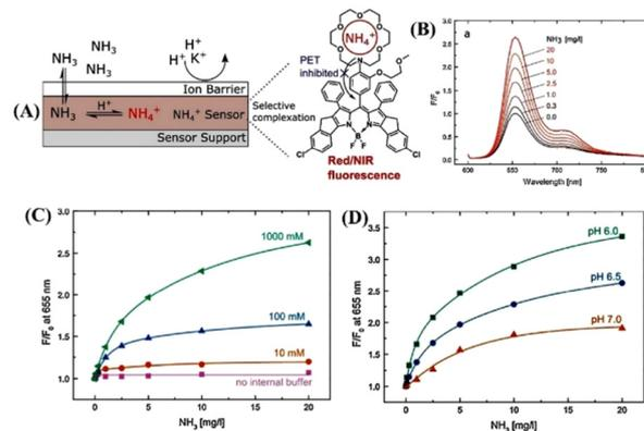
**Fig. 12** (A) New fluoroionophore mechanism for sensing of  $\text{NH}_4^+$  ions. (B) Changes in fluorescence emission spectra of the sensor **18** membrane were measured at different  $\text{NH}_3$  concentrations. (C) Calibration curves of the sensing materials with different buffer capacities. (D) Calibration curves of sensor **18** with different pH values of the internal buffer. Reprinted with permission from ref. 75. Copyright 2018 Elsevier.
