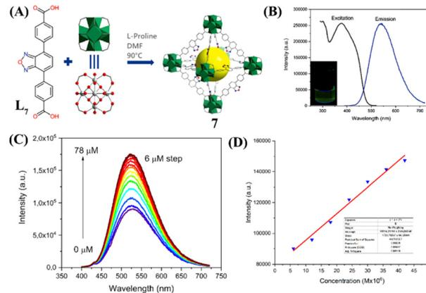
Fig. 4 (A) Synthesis of sensor LMOF 7 from ligand  $L_7$  and Zr(IV); (B) Excitation and emission spectra of 7 were measured in  $\text{H}_2\text{O}$  (inset: photographs of 7 in  $\text{H}_2\text{O}$ ); (C) Changes in fluorescence emission intensity for 7 upon the gradual addition of aqueous  $\text{NH}_3$ . (D) Linear fit for the  $\text{NH}_3$  concentration–intensity correlation. Reprinted with permission from ref. 51. Copyright 2022 Royal Society of Chemistry.
