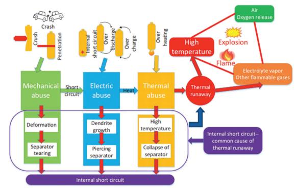
Fig. 11 Schematic illustration of LIB fire accidents.
