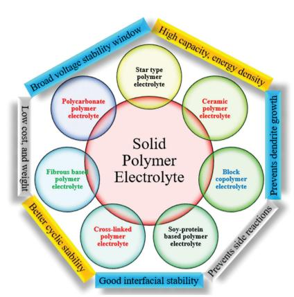
Different types of solid polymer-based electrolytes and their corresponding performances.
