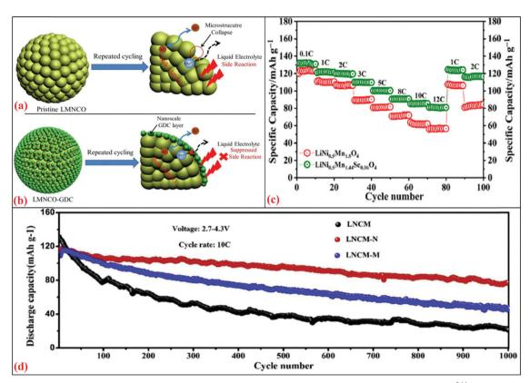
Fig. 8 Schematic illustrations of (a) pristine LMNCO interfacial side reactions with liquid electrolyte after repeated cycling<sup>244</sup> and (b) GDC coating layer acts as a protection layer to suppress the unwanted interfacial side reactions after repeated cycling. 245 (c) Rate capability for LNMO and LNMSO cathode for 0.1–12C. (d) Cycling performances for LNCM, LNCM-N, LNCM-M at C-rate of 10C. 246 Reproduced with permissions from Elsevier. 244–246
