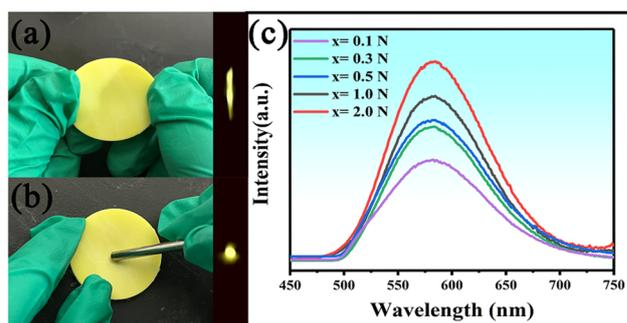
Fig. 6 (a) The image of a tensile test on  $\text{Ca}_{1.8}\text{Sr}_{0.2}\text{BO}_3\text{Cl}:\text{Eu}^{2+},\text{Dy}^{3+}$ ; (b) the image of the sample with an applied force of 2 N; (c) the ML spectra of  $\text{Ca}_{1.8}\text{Sr}_{0.2}\text{BO}_3\text{Cl}:\text{Eu}^{2+},\text{Dy}^{3+}$  under different force.
