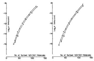
Fig. 9 (Left) Conductivity at 293 K for lysozyme, soaked in  $H_2O$  before and (Right) soaked in  $D_2O$ . Open Circles are for  $H_2O$  hydration data and open squares for  $D_2O$  data. Used with permission from J. Behi *et al. Int. J. Quantum Chem.*, 1982, **22**, 367–374. © 1982 John Wiley & Sons, Inc.<sup>22</sup>
