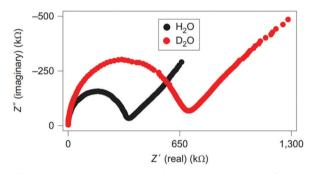
Fig. 10 Nyquist plots for reflectin films hydrated with H<sub>2</sub>O vs. D<sub>2</sub>O (labelled). Reprinted by permission from Springer Nature Customer Service Central GmbH: Nature, Nat. Chem., 6, 596–602, "Bulk protonic conductivity in a cephalopod structural protein", D. Ordinario et al. Copyright (2014).<sup>25</sup>
