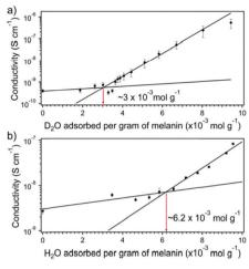
Fig. 11 (A) Conductivity of melanin with D<sub>2</sub>O content. (B) Conductivity of melanin with H<sub>2</sub>O content. Red arrows (with values) indicate the upturn in the conductivity at a critical amount of water content. Reprinted with permission from S. B. Rienecker et al. J. Phys. Chem. B, 2015, 119, 14994-15000. Copyright 2015 American Chemical Society. 46
