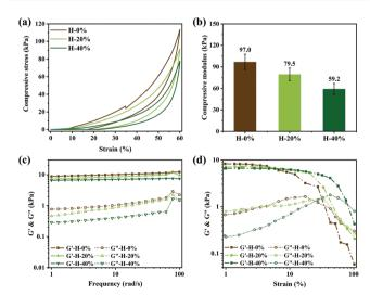
Fig. 5 (a) Compressive stress-strain curves and (b) modulus of H-0%, H-20%, and H-40%. Rheological behavior of H-0%, H-20%, and H-40% during (c) oscillatory frequency sweep and (d) oscillatory strain sweep.
