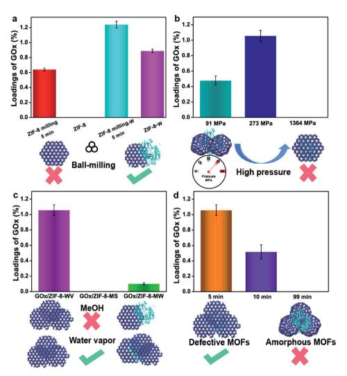
Fig. 2 Exploration of the several factors influencing the encapsulation of enzymes. (a) Loadings of enzymes adsorbed on ZIF-8 with or without premilling treatment. The loadings of enzymes adsorbed on ZIF-8 with or without premilling through PISA after soaking in water for 24 h. (b) Loadings of enzymes in ZIF-8 through PISA with different pressures. (c) Loadings of enzymes in ZIF-8 through PISA with different premilling time.
