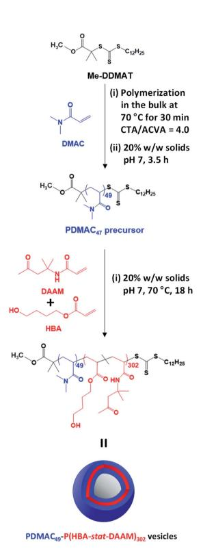
Scheme 1 Reaction scheme for the synthesis of the PDMAC $_{49}$  precursor via RAFT aqueous solution polymerization of DMAC at 70 °C using a Me-DDMAT RAFT agent and an ACVA initiator. This PDMAC $_{49}$  precursor was subsequently chain-extended via RAFT aqueous dispersion copolymerization of a binary mixture of 80 mol% HBA and 20 mol% DAAM to produce PDMAC $_{49}$ -P(HBA-stat-DAAM) $_{302}$  vesicles at pH 7.
