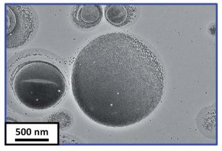
Fig. 4 Representative TEM images recorded for DS-ADH crosslinked PDMAC<sub>49</sub>-P(HBA-stat-DAAM)<sub>302</sub> vesicles prepared at a copolymer concentration of 5.0% w/w in the presence of a 20% w/w aqueous dispersion of silica nanoparticles (a) before and (b) after ten centrifugation–redispersion cycles to remove excess silica nanoparticles.
