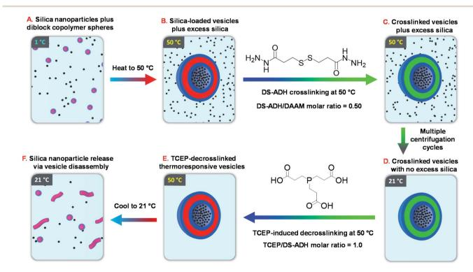
Fig. 1 Schematic overview of the six stages involved in the encapsulation and release of silica nanoparticles using a thermoresponsive 'shape-shifting' PDMAC $_{56}$ -P(HBA-stat-DAAM) $_{254}$  diblock copolymer.
